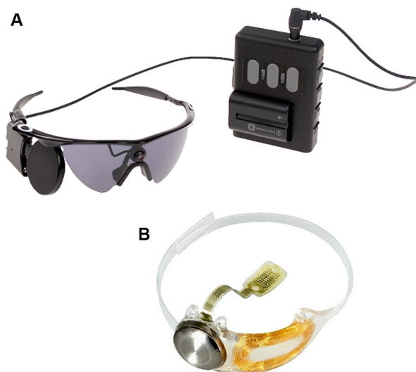
Fig. 3. (A) The external components; glasses (left) and video processing unit (right) of the Argus II implant. (B) The ocular components of the Argus II implant, including a scleral band, internal coil (for power and data transfer) and the electrode array which is attached to the epiretinal surface with a tack. Images courtesy of Second Sight Medical Products, USA.
