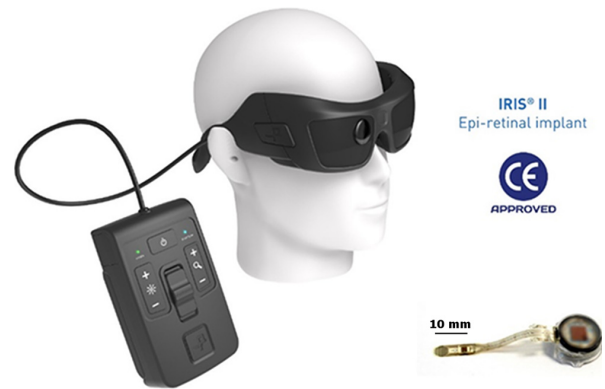
Fig. 4. The glasses and video processing unit (left) and ocular components (right) of the Iris II epiretinal implant. Images courtesy of Pixium Vision, France.
